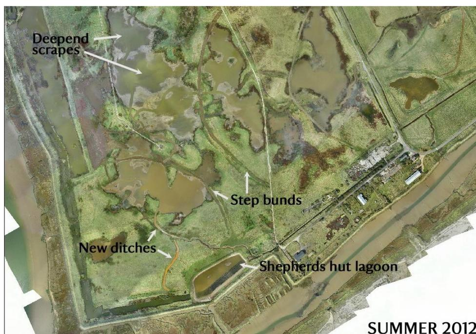
**Figure 3.** Aerial photograph of the south-west of Airfield Marsh, showing the shallow water pools and water control structures (earth bunds, ditches, and water storage lagoon).
