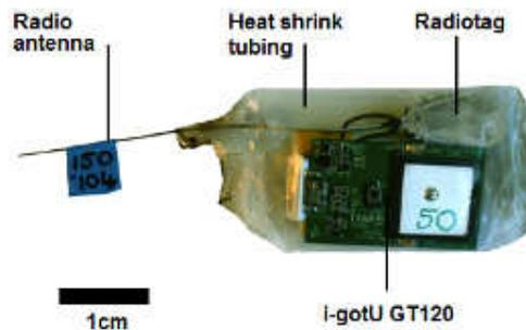
**Figure 1.** Custom made radio- and GPS-tag containing a TW-4 radio-transmitter with thermistor mortality sensor (Biotrack Ltd., Dorest, UK) and a deconstructed i-gotU GT-120 travel and sports GPS logger (MobileAction, Taipei, Taiwan) sealed inside heat shrink tubing to create a 40 x 20 mm, 17 g watertight unit.
