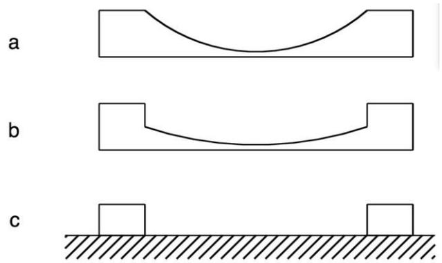
**Figure 2.** Cross section of three nest form shapes.
