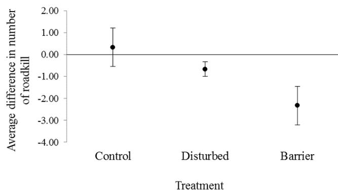
**Figure 3.** The average difference in number of roadkill counted in two 20-day periods occurring before and after the application of low-level roadside fencing to direct small terrestrial vertebrates to underpasses (culverts). Each treatment was applied to three 400 m segments of road (total 1.2 km) during February 2015. Error bars represent standard error.
